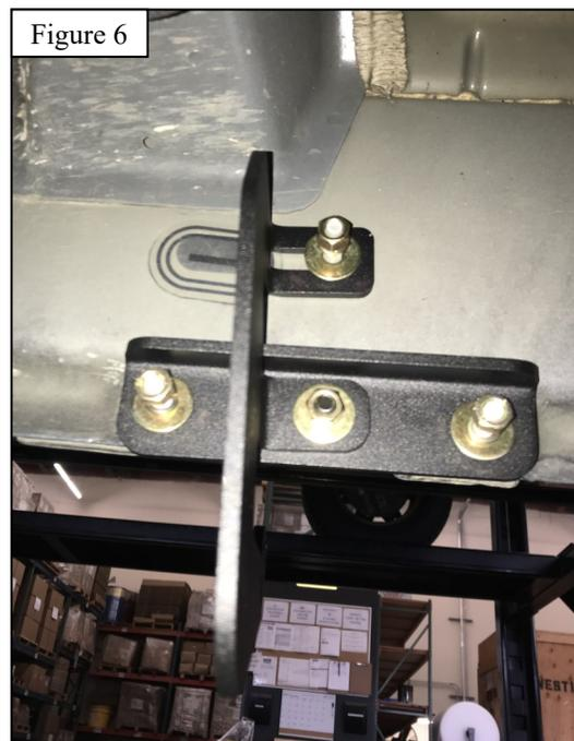
6. At the front passenger mounting location, loosely install the Mounting Bracket Base (Item 7) with preassembled Passenger Front Mounting Bracket (Item 4).
